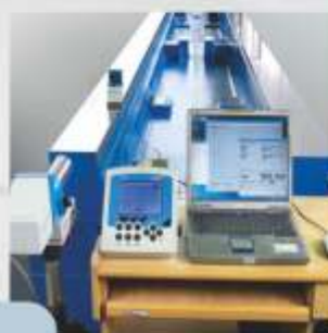
Straightness inspection with collimator
